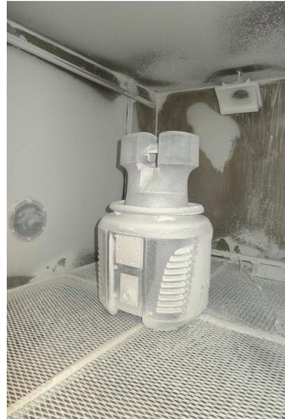
Fig. 11 APDIS after IP5X test.
