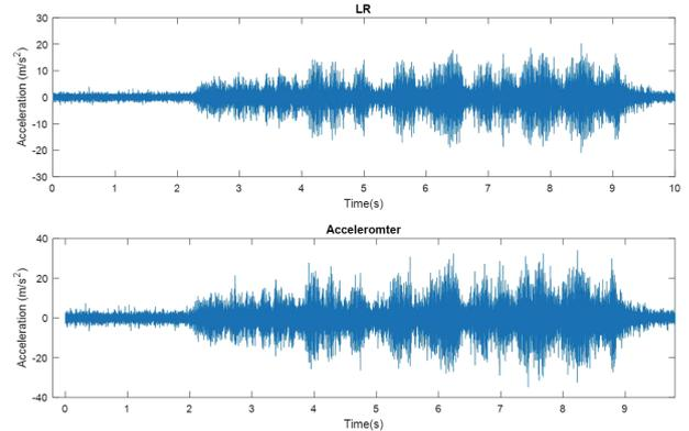
Fig. 14 Comparison of APDIS and conventional accelerometer.
