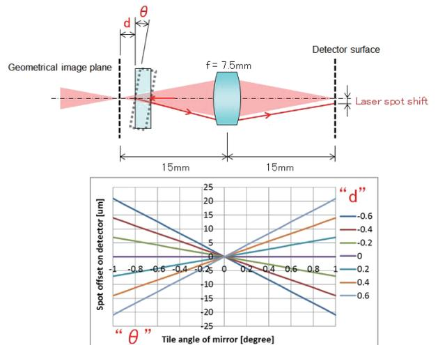
Fig. 4 Sensitivity of the mixing optics to misalignment.
