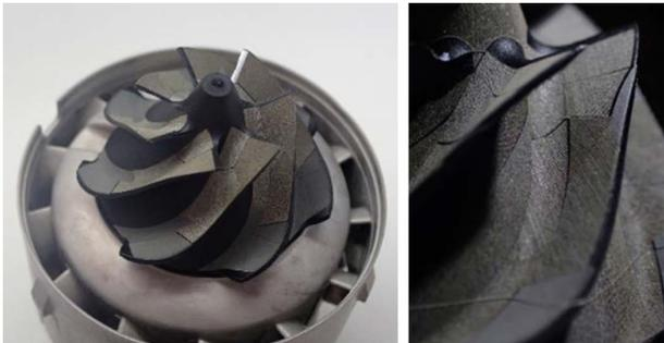
Fig. 5 Riblet processing on a 3D curved surface
