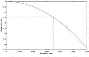
Fig. 5 Laser Radar signal loss due to beam shift.
