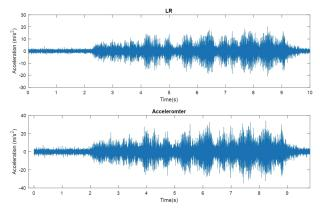
Comparison of APDIS and conventional accelerometer. Fig. 14
