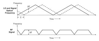
Fig. 1 Laser optical frequency and heterodyned RF signal of coherent laser radar.
