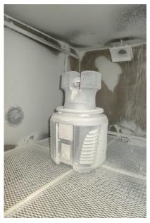
Fig. 11 APDIS after IP5X test.
