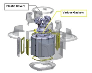
Fig. 10 Exploded view of external covers and various custom gaskets.
