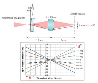
Fig. 4 Sensitivity of the mixing optics to misalignment.
