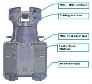
Fig. 9 APDIS cross-section showing various interfaces.
